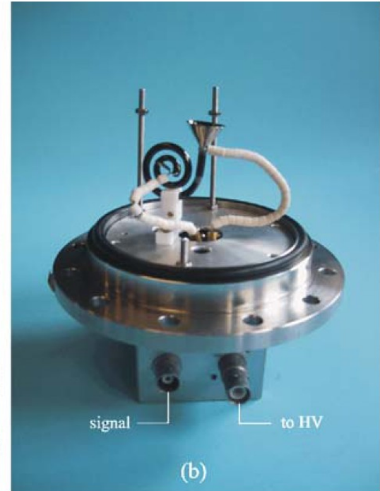
Figure 3. (a) View of the inside of the ILEEMS measuring chamber from the entry port for the cryostat. On the left is the cone with Be window for the incident radiation. The channeltron is closely above it. On top of the cubic chamber on the outside is the voltage divider. (b) Picture of disassembled top plate showing the mounting of the channeltron.
